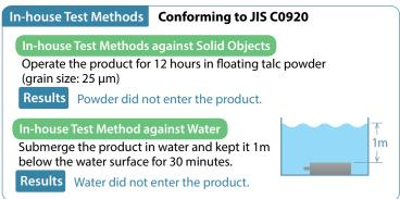
The splash-proof performance has been measured only with regard to water. Protection against coolant, cleaning solution, etc., is not guaranteed. If you wish to use your product in an environment where it may come in contact with coolant, consult IAI beforehand.
