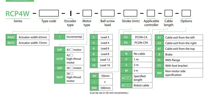
The settings for motor type, ball screw lead, stroke and options vary from one model to another. For details, check the specifications for each model.
