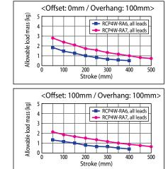
Allowable load calculation conditions: Load mass corresponding to a guide traveling life of 5,000 km, considering moments generated by acceleration/deceleration. (Acceleration: 1 G / Speed: 500 mm/s)
