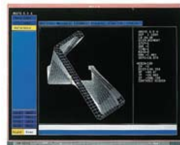
Deformation of a competitor's base structure under the same amount of force.
