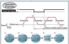
Acceleration and Deceleration Can Be Set Differently With ROBO Cylinders, acceleration and deceleration are set in the position data table. Since acceleration and deceleration can
