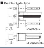
\* Single-guide actuators cannot receive any load other than in vertical direction.
