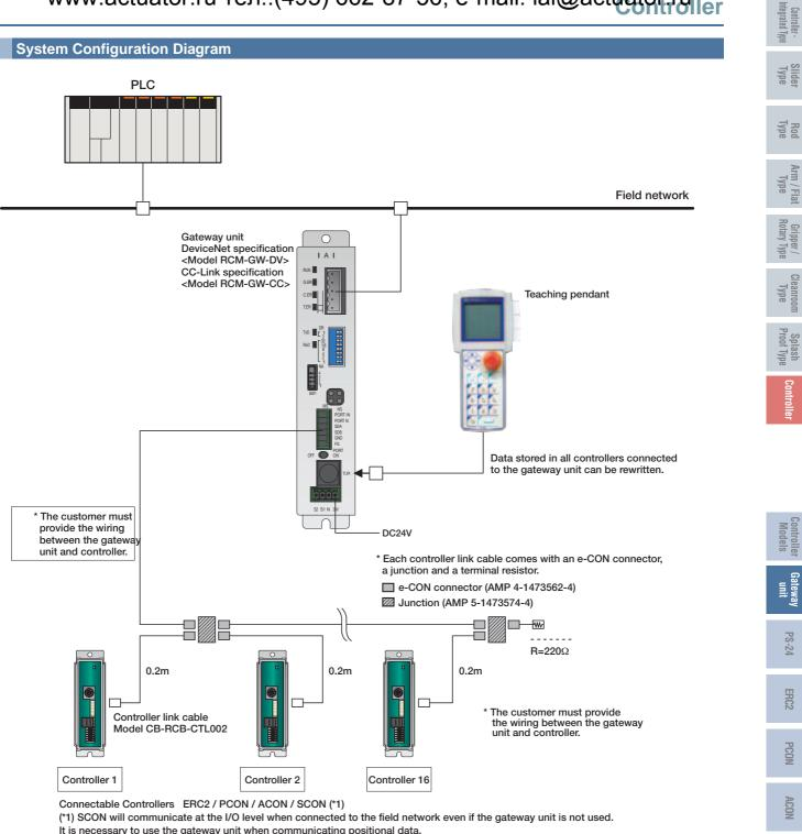
It is necessary to use the gateway unit when communicating positional data.
