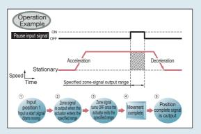
No Microvibration at Stopping (ERC2/RCP2) ROBO Cylinders do not generate microvibration associated with conventional servo motors, which makes them ideal for measurement systems equipped with a camera, etc.
