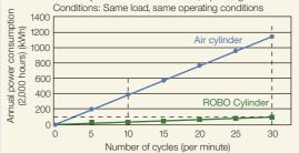
Two new functions were added to enhance the energy-saving features of ROBO Cylinders that already offer higher energy efficiency than air cylinders.
