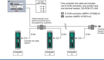
The diagram shows only serial communication connection.
