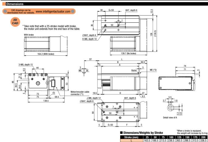
(\*1) An integrated motor/encoder cable is provided. (Refer to P. 34.) (\*2) The slider will move to the ME after home return, so pay attention
