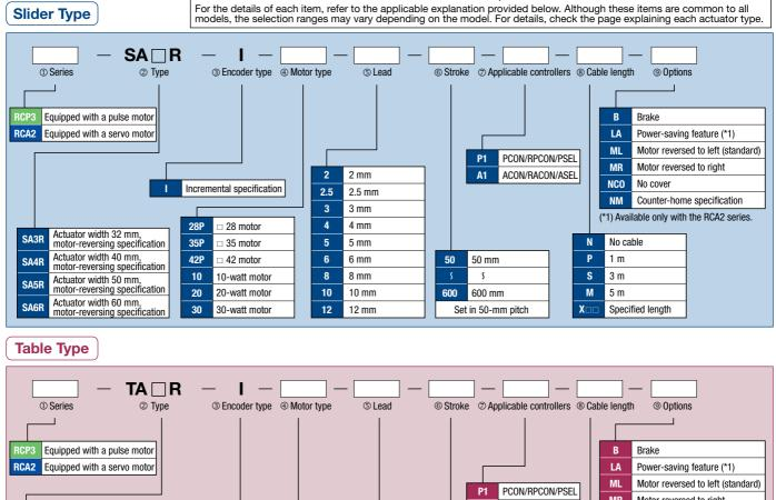
The model names of RCP3/RCA3 actuators consist of the items specified below.
